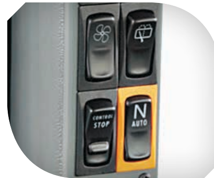
Electronic engine control enables versatile cruise controls.
