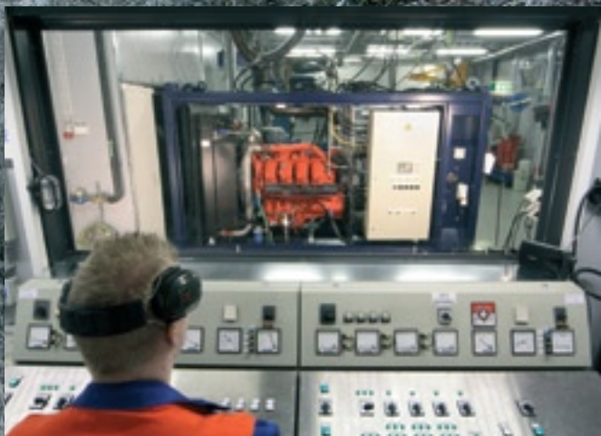
Each genset and pump set is thoroughly tested and load test run before delivery with modern genset test facility
