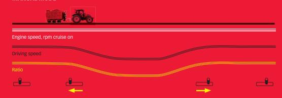
Manual mode can be selected in A and B work ranges. The transmission ratio is controlled solely by driver using the CVT lever. Suitable especially for harvesting tasks that require specific speeds for different conditions and crops.
